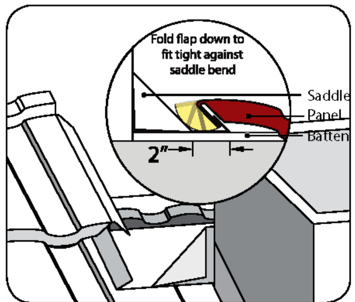
Flatten the back flange of the panel intersecting the top of the protrusion.
